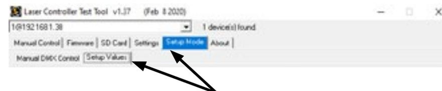
Adjust the settings (besides the laser output, the little window in the bottom right of the ‚Setup Value‘ tab will display the changes, too) and then store them to the ShowNET laser mainboard with a click on ‚Save‘. The laser output will flash three times to confirm that the changes have been saved.
