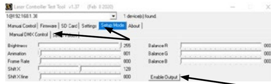
Select the tab ‚Setup Mode‘ -> ‚Setup Values‘ as shown in the picture below:
